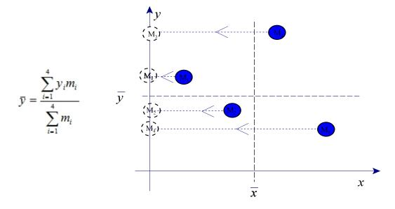
The numerator of the expression for both the x and y coordinates of the center of mass of the mass system is the sum of the moments of masses about the y-axis and the x-axis respectively.
