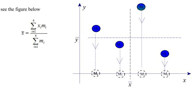
And similarly, translating the masses parallel to the x axis allows to compute  $\bar{y}$
