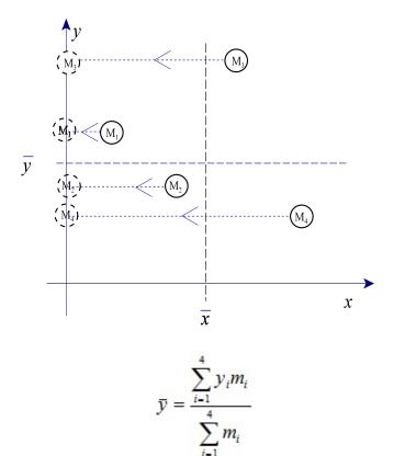
The numerator of the expression for both the x and y co-ordinates of the center of mass of the mass system is the sum of the moments of the masses about the x-axis and the y-axis respectively.
