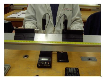
In the photograph above, glider 1 (on the left) has the only flag. Its flag triggers the left photogate for the glider's time before the collision. Then very soon after the collision, the same flag on glider 1 will trigger the right photogate. You can see how close the two photogates can be to one another (which is desirable) when using this method.
