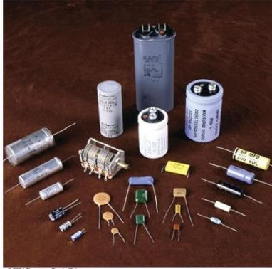
What is a capacitor and how can a capacitor store energy? A capacitor can be formed by two conductors separated by an insulator (vacuum, plastic, wax paper). The simplest form of a capacitor is the parallel plate capacitor.
