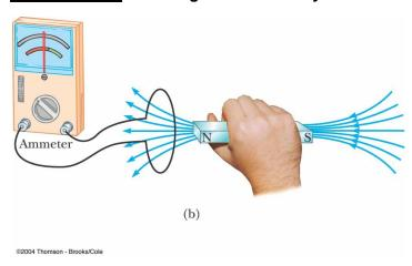
When the magnet is held stationary, there is no induced current in the loop, even when the magnet is inside the loop.
