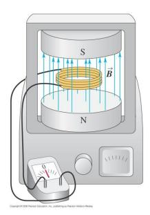
When the coil is rotated in the uniform B-field, an induced current and thus an induced EMF is also set up in the loop.
