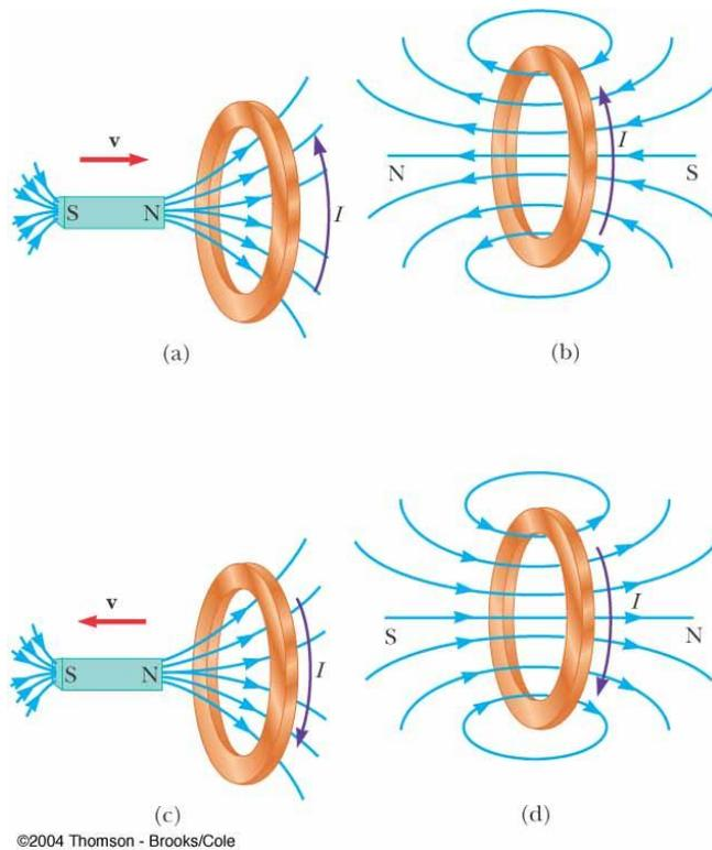
(a) When the magnet is moved toward the stationary conducting loop, a current is induced in the direction shown. (b) This induced current produces its own magnetic field directed to the left that counteracts the increasing external flux. (c) When the magnet is moved away from the stationary conducting loop, a current is induced in the direction shown. (d) This induced current produces a magnetic field directed to the right and so counteracts the decreasing external flux.
