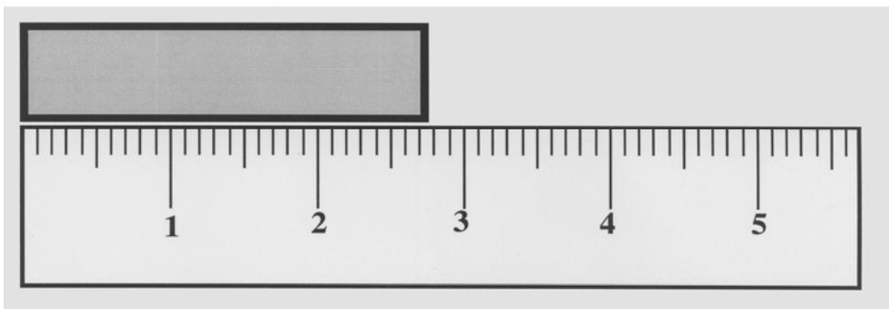
The ruler is incremented in units of centimeters (cm). The smallest scale division is a tenth of a centimeter or 1 mm. Therefore, the uncertainty  $\Delta x = \text{smallest increment}/2 = 1\text{mm}/2 = 0.5\text{mm} = 0.05\text{cm}$ . Note that a measurement made with this ruler must be stated to a tenth
