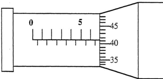
In the figure to the left, notice the main scale which is marked with a 0 and a 5. These indicate millimeters. Below the main scale are marks at the half way points between mm marks. These 1/2 mm marks are present because one revolution of the thimble moves the thimble only 1/2 mm down the barrel.
