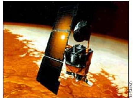
The units mismatch prevented navigation information from transferring between the Mars Climate Orbiter spacecraft team in at Lockheed Martin in Denver and the flight team at NASA's Jet Propulsion Laboratory in Pasadena, California.
