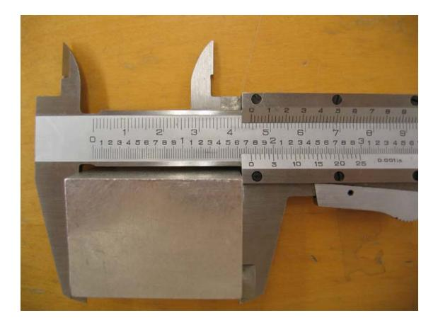
Note that the zero line on the vernier scale falls between the 4.4 cm and 4.5 cm mark on the main scale. Thus, the first significant digits are 4.4 cm. The remaining two digits are obtained by noting which line on the vernier scale (0,2,4,6,8) coincides best with a line on the main scale. Looking closely at the picture below indicates that the 46 line lines up the closest. Therefore, the reading is 4.446 cm. Or in standard form 4.446 cm ± 0.001 cm.
