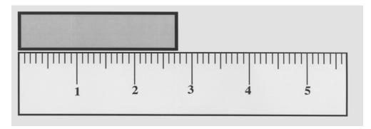
The ruler is incremented in units of centimeters (cm). The smallest scale division is a tenth of a centimeter or 1 mm. Therefore, the uncertainty  $\Delta x = \text{smallest increment}/2 = 1\text{mm}/2 = 0.5\text{mm} = 0.05\text{cm}$ . Note that a measurement made with this ruler must be stated to a tenth of a centimeter since the uncertainty is stated to a tenth of a centimeter. In the example above, the length of the object would be stated as  $x = 2.77 \text{ cm} \pm 0.05 \text{ cm}$ .
